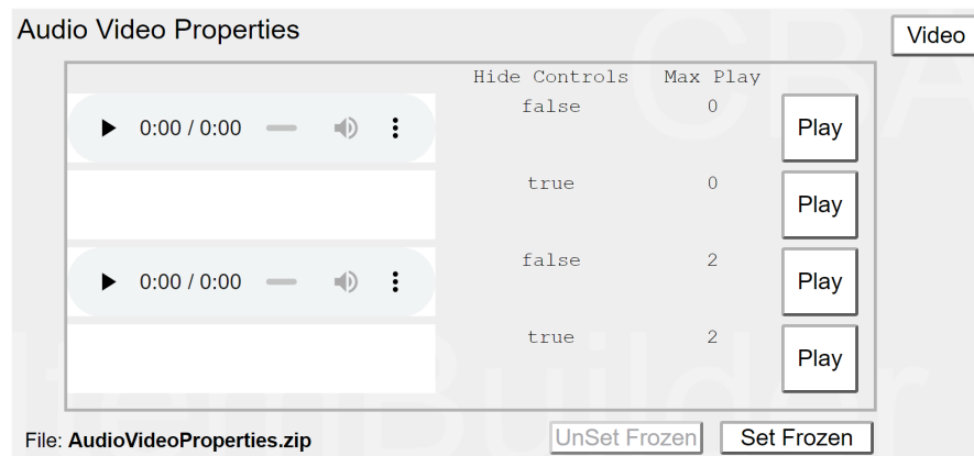
FIGURE 3.120: Item illustrating the use properties Hide Controls and Max Play of Audio and Video components ( html|ib ).
